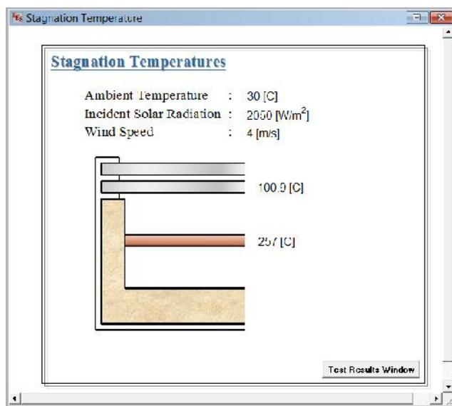
Figure 14 Steady state stagnation temperatures
