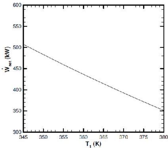
Figure 8 effect of the ORC pump inlet temperature on the electrical power
