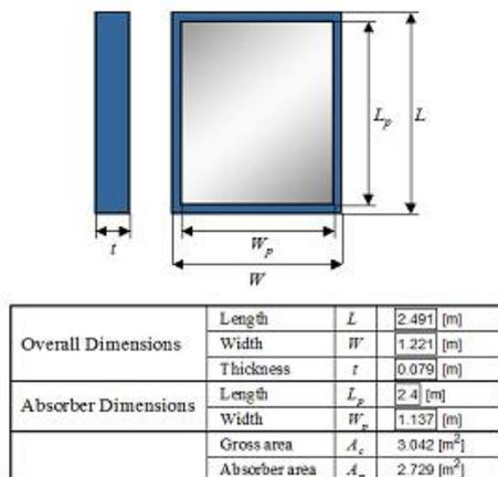
Figure 1 Collector Dimensions
