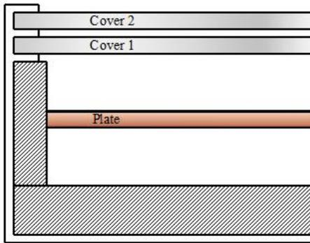
Figure 3 Cover and Plate of the solar flat plate collector
