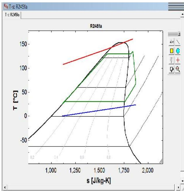
Figure 10 Organic rankine cycle with R245fa as working fluid
