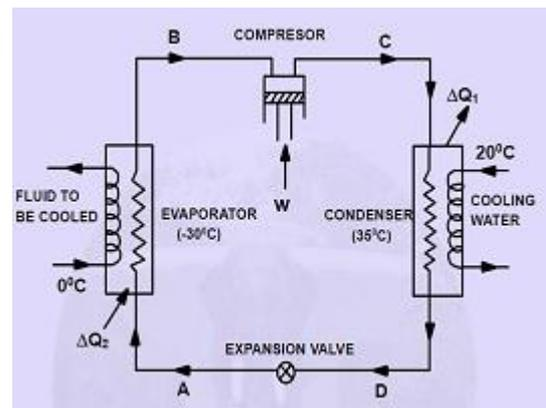
Figure 09 A simple Vapour Compression refrigeration cycle
