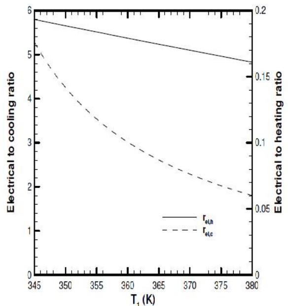
Figure 15 effect of the ORC pump inlet temperature on the electrical to heating
