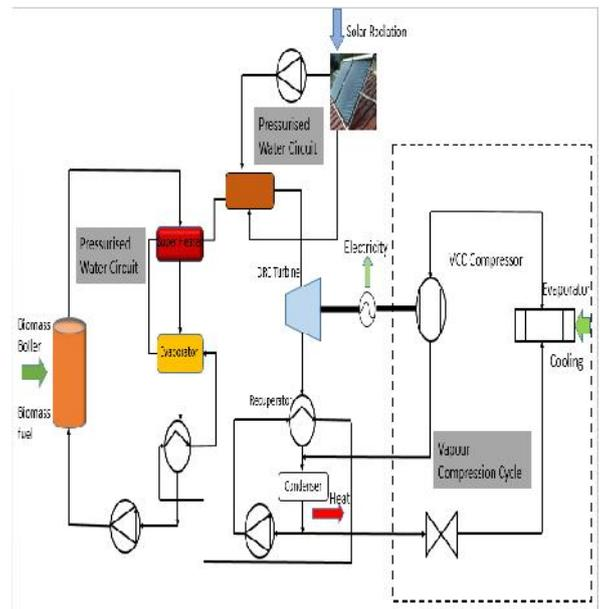
Figure 2 The proposed system for Solar-Biomass Hybrid trigeneration system using ORC-VCC
