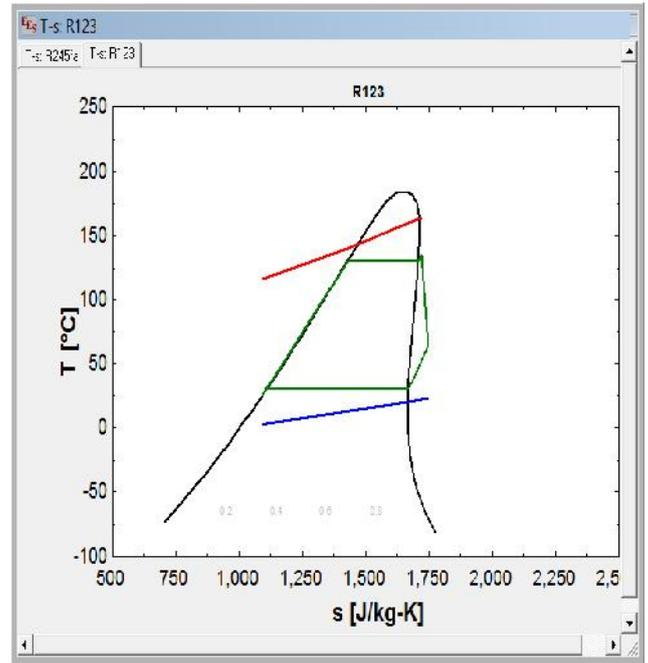
Figure 11 Organic rankine cycle using R123 as working fluid
