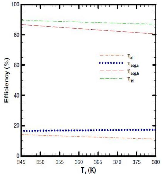
Figure 14 effect of the ORC pump inlet temperature on the efficiency at  $P_s$  at 2000 Kpa
